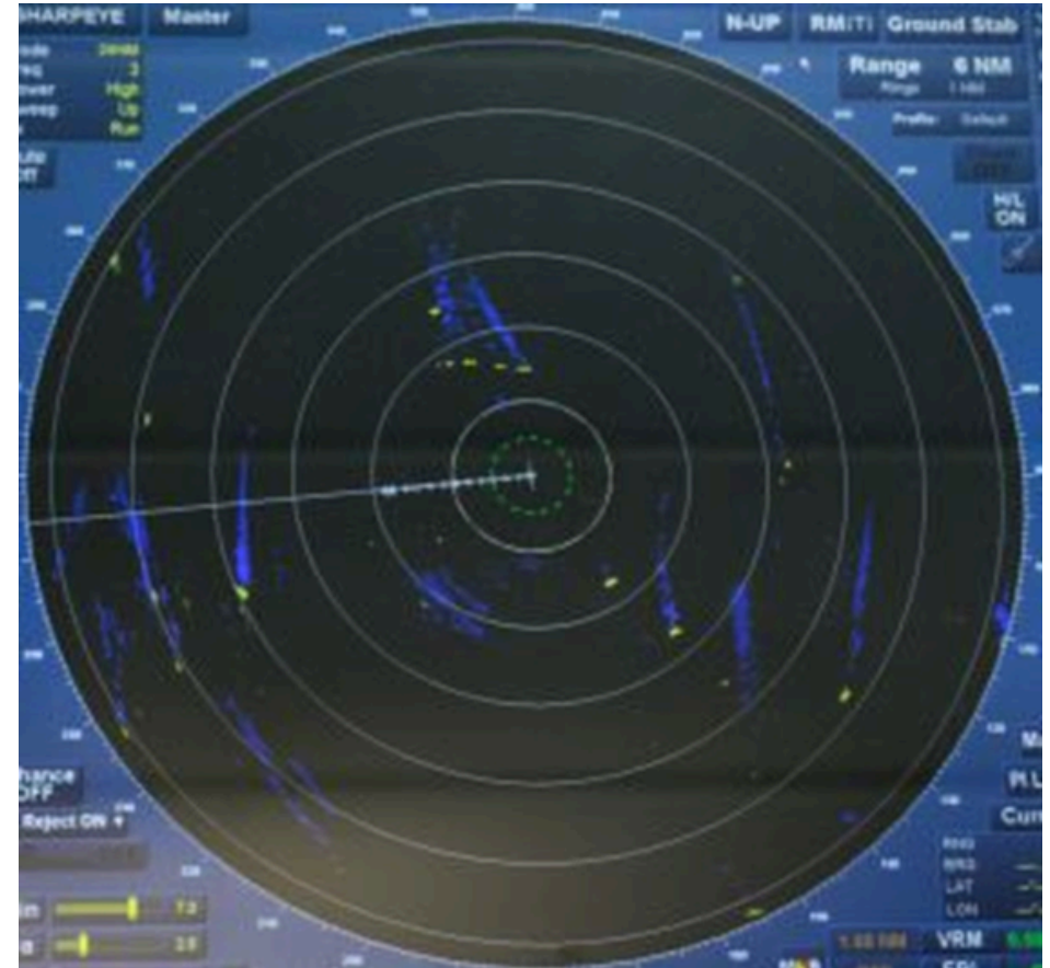
Woodpigeon flocks on the CEFAS Endeavour radar. Each yellow target on the screen is a flock and the blue trail shows the direct of travel (courtesy of Pete Howlett)
